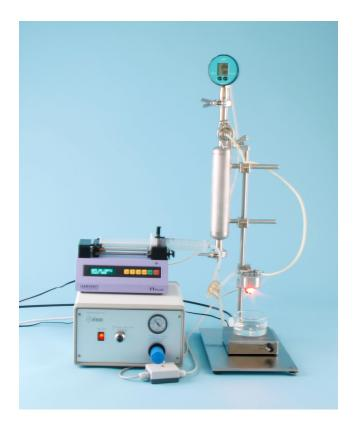
The exit orifice is placed centrally and in line with the needle exits. The input of a controlled pressure into the chamber gives rise to a pressure gradient across the exit orifice and generates an aerodynamic flow field.
