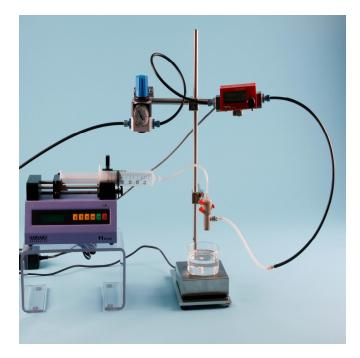
An easy way for production of small polymer beads in a controllable manner is the use of a coaxial bead generator. The basic principle of the instrument is the use of a coaxial air stream to blow droplets from a needle tip into a gelling bath before they would fall due to gravity. The unit is equipped with two connections, one for the hose which provides the alginate gel, and the other connection is aimed for an air hose.
