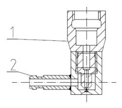
The product flows through the product nozzle (1) which is placed in the specially constructed pressure chamber (2).
